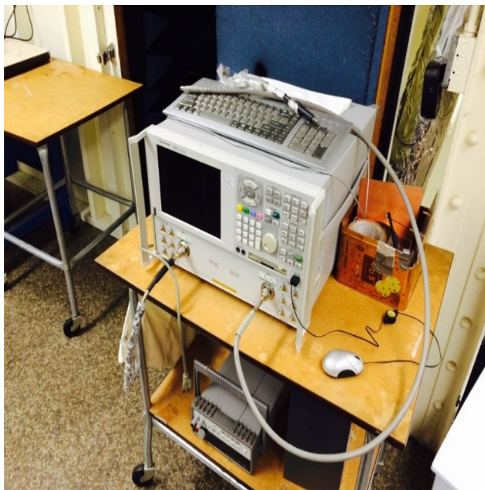
Fig.3.1 Agilent Network Analyzer used to collect and analyze data
