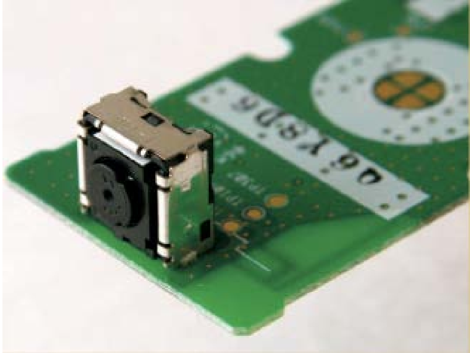
Fig.2.2 IR camera chip .Integrated multi-object tracking minimizes wireless data transmission
